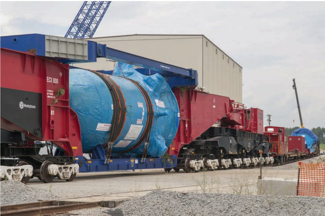
Summer Unit 2—Reactor Vessel delivery, AP1000, June 2013, United States (SCANA).
