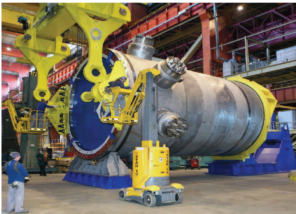
Flamanville unit 3—Preparation for hydraulic test of the reactor vessel, EPR, August 2010 (AREVA, SIRAND Tracy).
