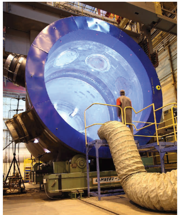
Flamanville unit 3—Reactor vessel for site, Welding of the final weld, manufacturing plant, EPR, Chalon St Marcel, France, June 2010 (AREVA, SIRAND Tracy).
