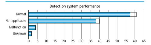
The "Not applicable" reporting frequency is relatively high. This results mainly from situations of fires detected early and subsequently extinguished quickly by plant personnel available in the fire area, and fires at locations without detectors, for example outside buildings. Excluding the "Not applicable" cases, the detection systems are considered to have performed normally in almost all real-demand situations.
