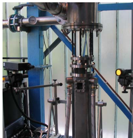
Figure 5: The test section and the PIV system
