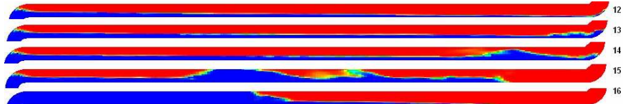
Figure 4: Volume fraction in upper pipe in simulations with Large-Interface model at different times (blue – water, red – steam).
