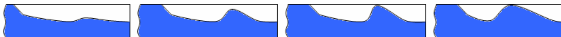
Figure 1: Schematic view of bubble entrapment and its condensation, from left to right: the wave appearance, the growth of the wave, the wave touches the wall and the entrapped bubble is shrinking due to condensation.
