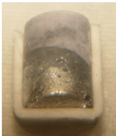
Liquid Cd cathode in Al 2 O 3 crucible after electrolysis
