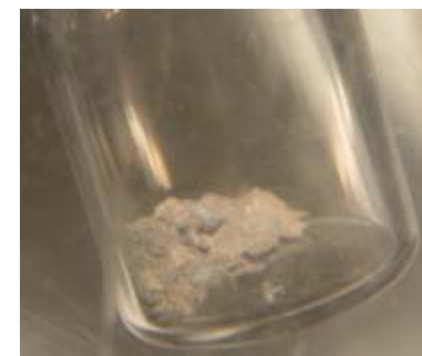
(U,Pu)N powder obtained by nitridation/distillation combined reaction
