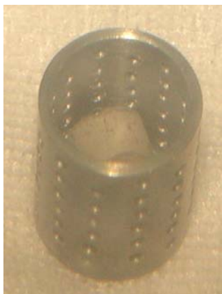
(U,Pu)N pellet in Mo crucible before electrolysis
