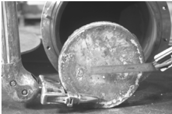
Metallic Waste Form from Electro-Chemical Processing
