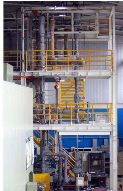
HELIOS : non-isothermal, flowing LBE Test
