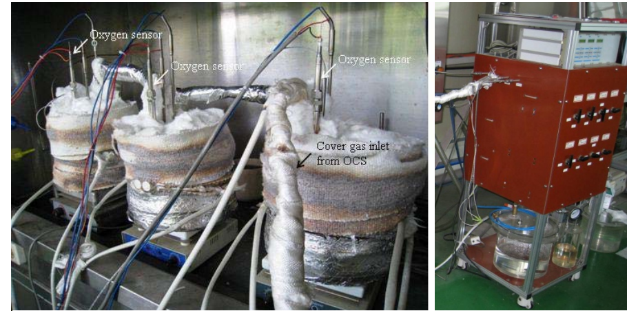
Static cells (left) and oxygen control system (right)
