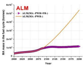
Big differences are observed between LWR open cycles and FRs closed cycles (up to one order of magnitude)
