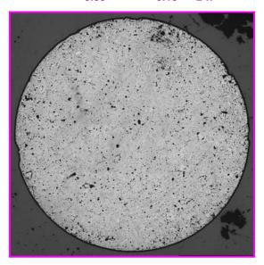
**Optimized microstructure with** tailored open porosity: 14 discs  $(U_{0.85},^{241}Am_{0.15})O_{2-x}$
