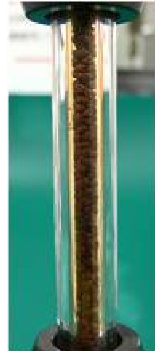
Column of the Fe adsorbent used in Mo separation tests
