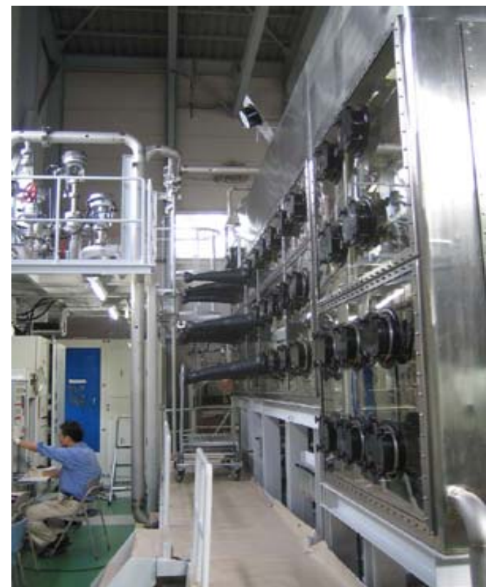
Ar atmosphere Large Glove Box
