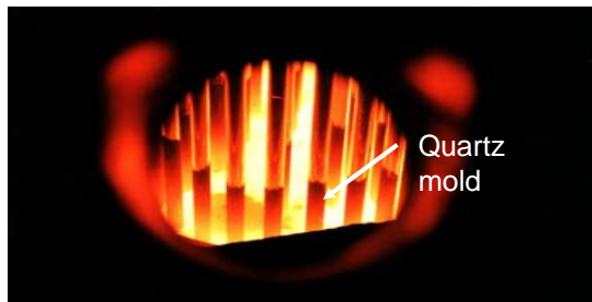
Inside view during casting
