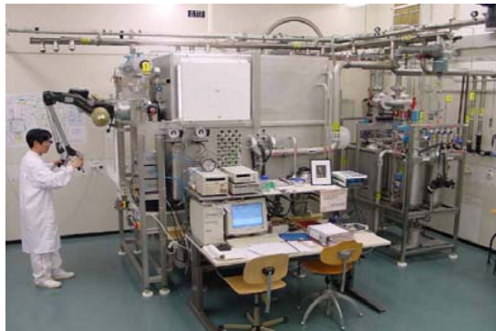
Caisson with high purity Ar atmosphere and manipulating operating system
