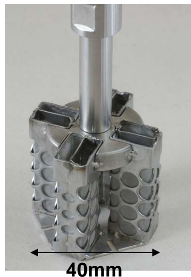
Reduction of MOX (55U-5Np-40Pu) was confirmed with small scale
