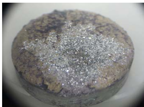
Cd ingot with U+Pu (Cd:120g, U+Pu:14.7g)
