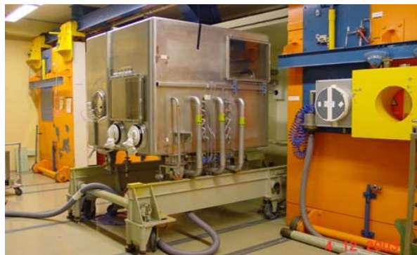
Dismantling and transfer to hot cell after experience with non irradiated TRU-containing material
