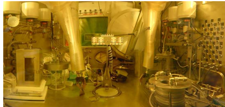
Set up of caisson in hot cell
