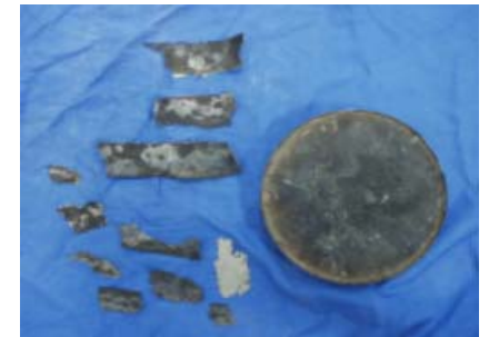
Heel and dross in crucible
