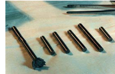
U-Pu-Zr-MA-RE* MA; Np, Am, Cm RE; Ce, Nd, Y, Gd (Fabricated by arc-melting)
