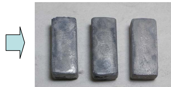
Reduction of \text{UO}_2 in larger scale was confirmed in ~100g scale
