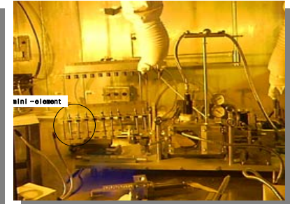
Remote Welding of Rod
