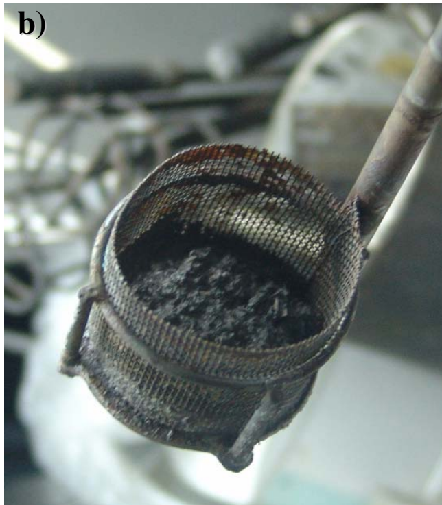
Self-scraped Uranium Dendrites
