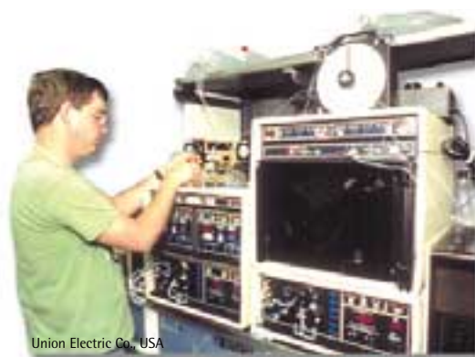
The health physics laboratory at Callaway nuclear power plant, in the United States, where environmental samples are measured for radioactivity.
