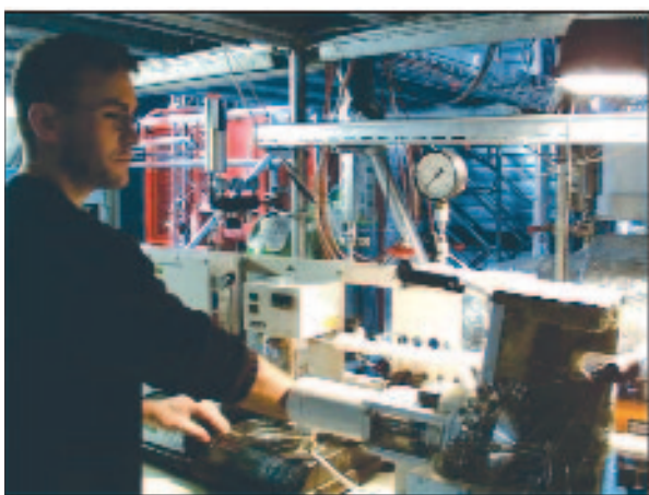
Measurement of local gas concentrations inside PANDA vessels and components (mass spectrometer) at the PANDA experimental facility in Switzerland.
