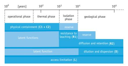
An example from ONDRAF of the four phases of the normal evolution of a repository for high-level waste and the corresponding long-term safety functions. The first two safety functions can each be subdivided into two sub-functions. For the "physical confinement" function, which aims to prevent any release of activity from the waste matrix, the two sub-functions are "water tightness" (C1) and "slow water infiltration" (C2).
