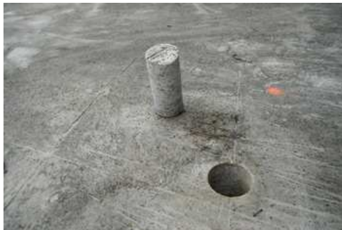
Core made of concrete containing C-14
