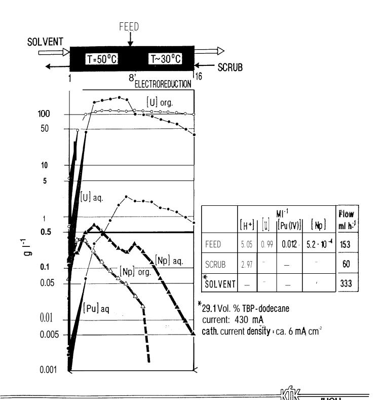
BEHAVIOR OF Np IN A MIXER-SETTLER BANK UNDER HIGH LOADING CONDITIONS (increased temperature and increased [HNO<sub>3</sub>] in the feed) AND USE OF ELECTRO - REDUCTION IN SEVEN STAGES OF THE SCRUB SECTION
