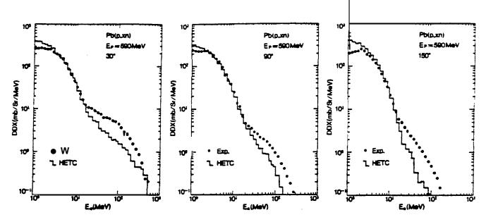
Figure 2: Double-differential cross sections for neutrons at 30, 90 and 150 degrees from a thin lead target for an incident proton energy of 590 MeV. The solid circles are the experimental data and the solid curves represent HETC calculations [12].
